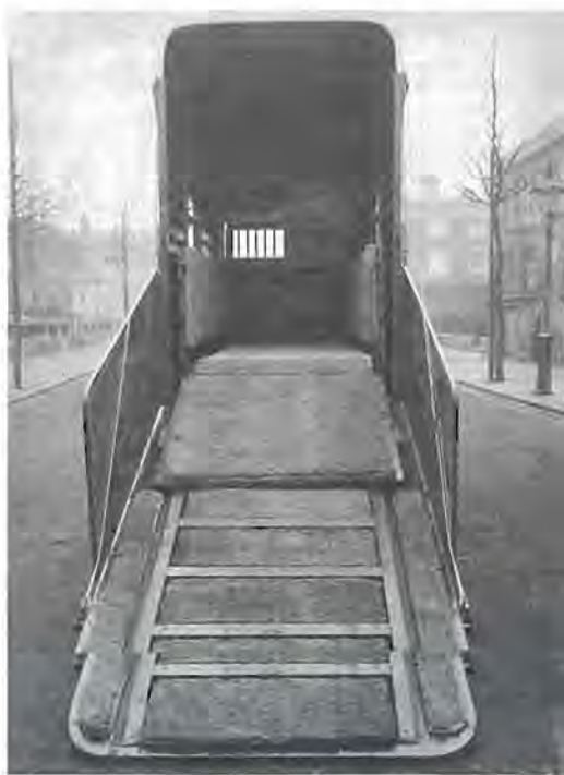
The 'Lonsdale' ambulance for two horses, built by Dennis Bros. at their factory in London, W10.
